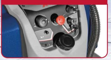
3 power stages for the suction motor in order to reduce its noise up to 67 dB.
