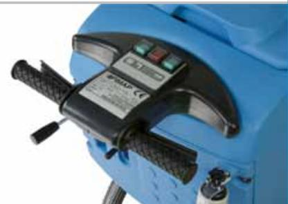
The shape of the instrument board, made of cast aluminium and injection moulded, facilitates machine control and guarantees the best visibility and safety of use
